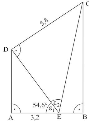
$$\begin{aligned}\cos(\varepsilon_1) &= \frac{\overline{AE}}{\overline{DE}} \\ \cos(\varepsilon_1) \cdot \overline{DE} &= \overline{AE} \\ \overline{DE} &= \frac{\overline{AE}}{\cos(\varepsilon_1)} \\ \overline{DE} &= \frac{3,2}{\cos(54,6^\circ)} \\ \overline{DE} &\approx 5,52 \text{ cm}\end{aligned}$$
